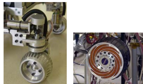
Fig.4. Typical modified wheel against the original wheel
